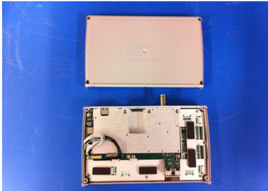
Figure 4-9. Back Cover Removed
