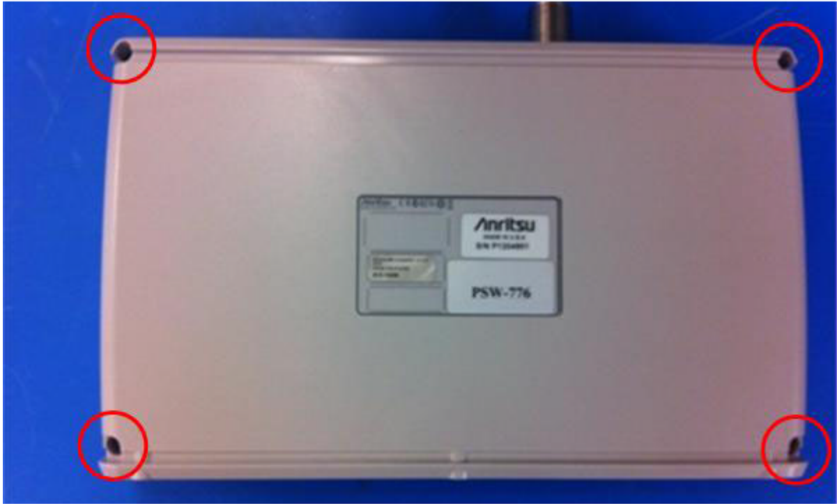
Figure 4-8. Place Unit Face Down and Remove Four Screws
