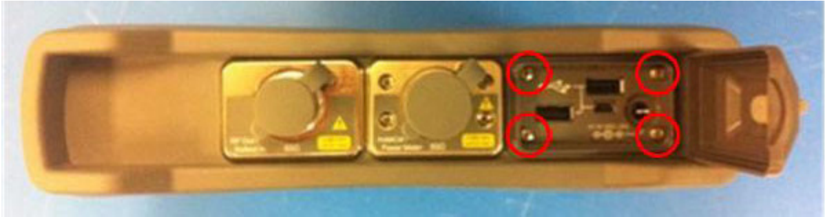
Figure 4-4. USB / Power Cover Removal
