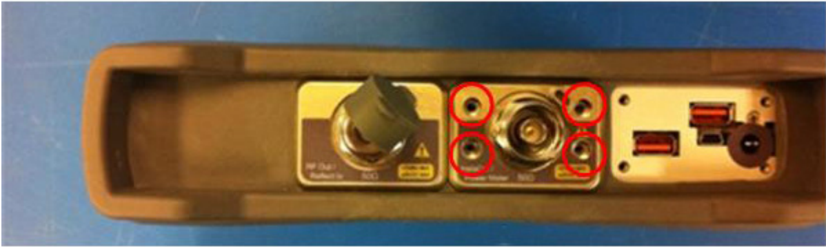
Figure 4-12. InstaCal / Power Meter Removal
