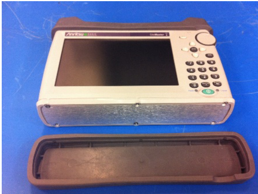
Figure 4-1. Bottom Bumper Removal
