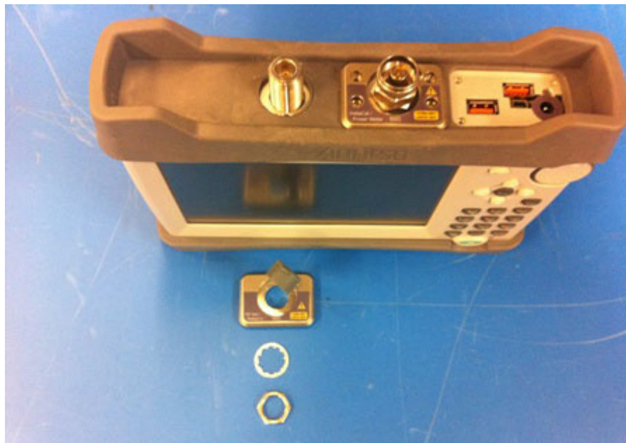
Figure 4-5. RF Out Mounting Plate Removed
