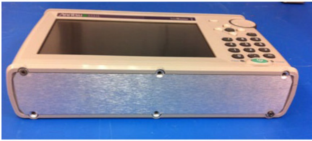
Figure 4-2. Battery Cover Removed
