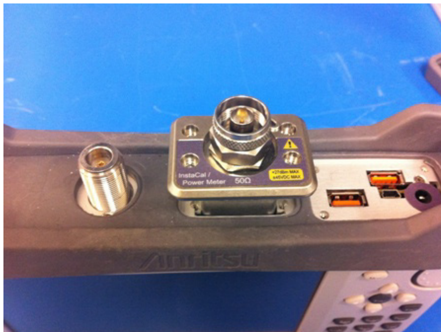
Figure 4-6. Remove 4 screws and InstaCal / PM Module
