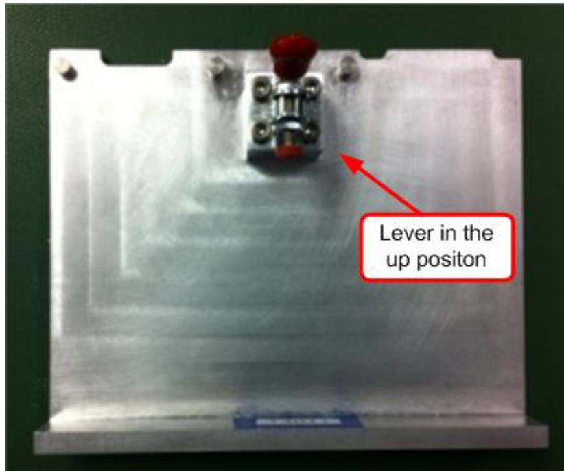
Figure 4-22. Test Fixture T4011 with Lever in Up Position
