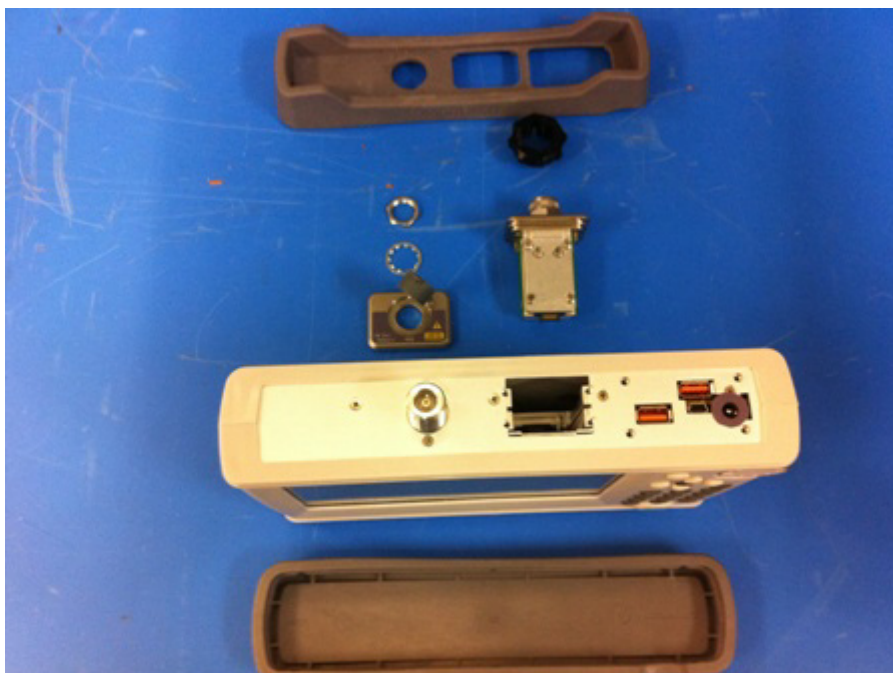
Figure 4-7. Both Bumpers, Batteries, Battery Cover, RF Out Mounting Plate and InstaCal/PM Module Removed
